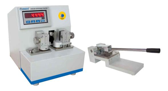
**Crease Stiffness Tester** is a multi-function stiffness tester, mainly used for measuring cardboard, color box (such as cigarette case cosmetic box) of the indentation force (that is, 90° crease of the rebound force), can also measure a variety of cardboard Bending stiffness is achieved on the same instrument with two measurements: 15° flexing Degrees and 90° crease stiffness.
